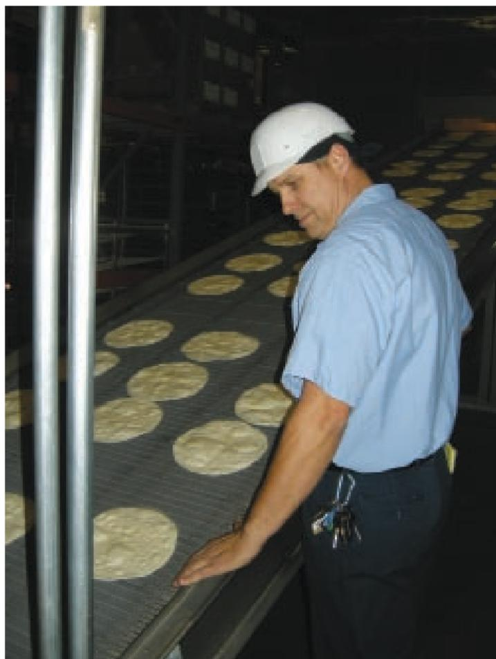
◀ Jim Fuller, production manager, inspects tortillas as they exit the oven where they bake for 22 seconds at 400°F.
